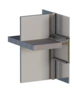
Acoustic board limiting sound transmission where curtain walls and internal partitions abut
