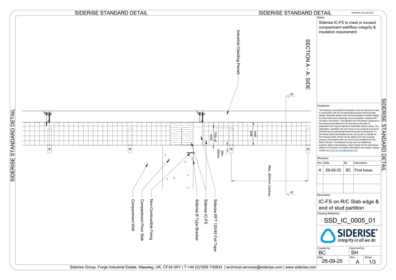
Siderise IC-FS to meet or exceed compartment wall/floor integrity & insulation requirement.
