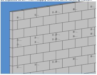
Depending on the size and thickness of Siderise ALS acoustic lining slab used, and the orientation, the number of fixings required will alter. The information in Table 1 is offered as guidance only.
