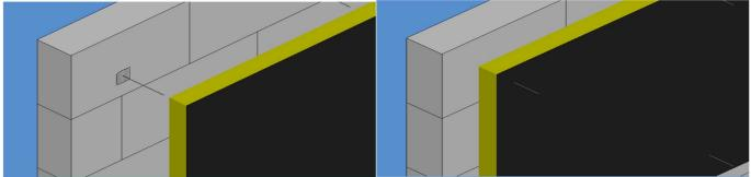
The second row would again start at the top of the treatment area, to the right of the 1st sheet, this should be continued as above, further rows would be fitted until complete treatment area is covered.
