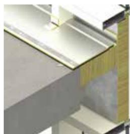
**SIDERISE AB** acoustic barrier overlay for use above the perimeter barrier firestop. Different grades are available to suit acoustics performance required. For guidance, tested performance for composite assembly:
