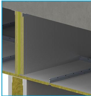
Fig 3. Head fixing with twin angle sections
