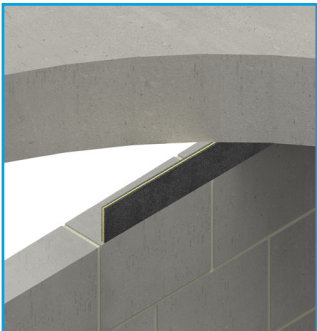
Fig 3. Deflection/Fire seal at top of wall
