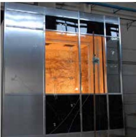
As a guide to performance a full curtain wall assembly was tested to BS EN 1364-3:2006 fire resistance test for non-load bearing elements achieving a performance of REI 30 with no issues regarding integrity or insulation. The assembly consisted of the following:
