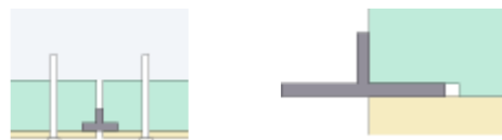
Figure 3. Shadow line Joint method
