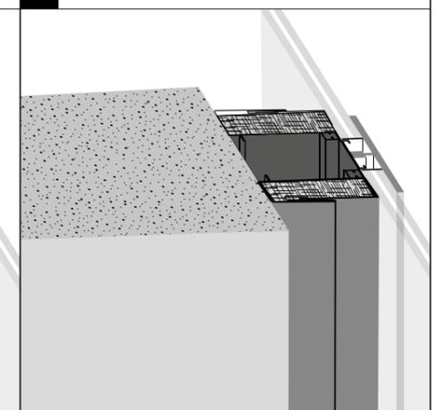
**10** Cut the male cover plate to the appropriate length to suit the treated area, using a hack-saw.
